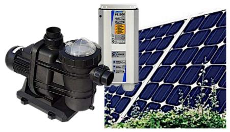
The LORENTZ pump uses a DC brushless motor for high efficiency and reliability, it is connected to a solar generator via a controller. The controller monitors the system, controls the pump speed and optimizes the amount of water pumped based on the power available.
